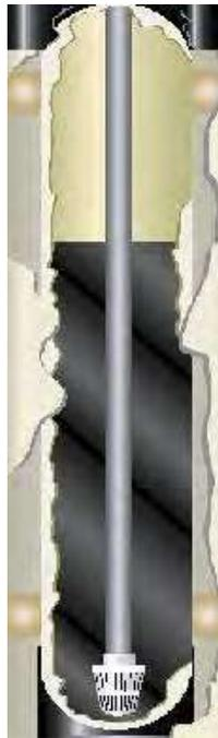
Typically it will center in an indentation in the bottom of the tank. Once it is centered, you will need to put duct tape over the tube to prevent media from getting in the tube during the fill procedure.
